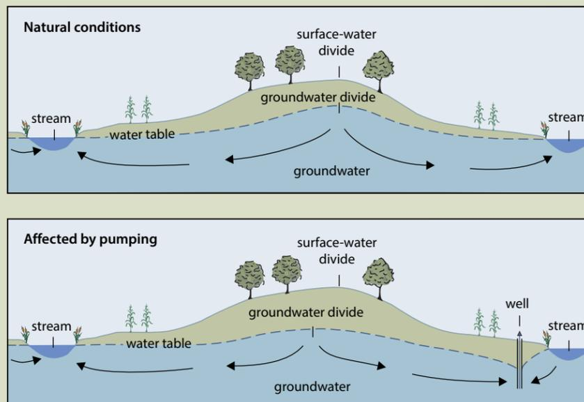
Figure 3. Groundwater flow under natural conditions and with pumping. Source: Adapted from USGS Water Resources Investigations Report 00-4008.
